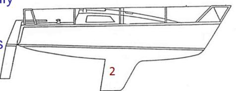
The keel provides ballast so that the boat doesn't turn over (capsize) when wind & waves apply pressure from the beam (or side) of the boat.
